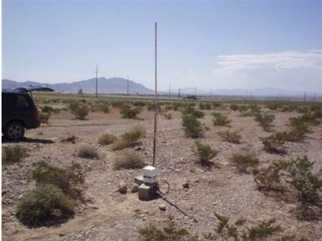
Figure 3-2. Sampler Mounting at Ground Level with the Sample Inlet at the Top of the Pole
